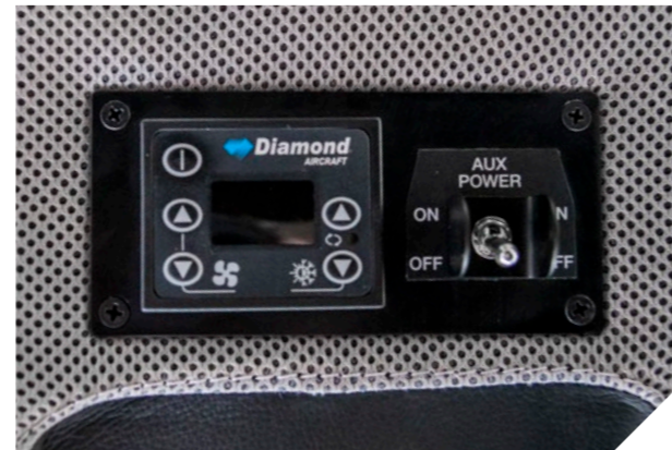
Air conditioning/RACC II system (powered by an additional alternator)
