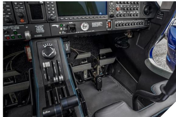
Electrically adjustable rudder pedals for pilot & co-pilot
